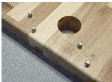
Insert the machine screws from the underside.
