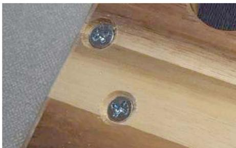
Countersink the BOTTOM sides of the mounting holes to recess the heads of the machine screws,
