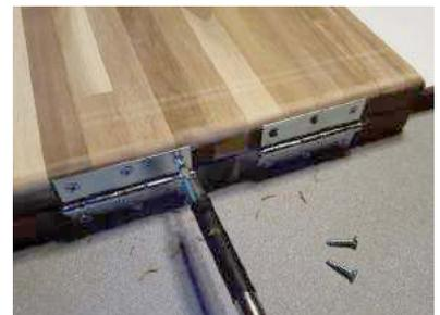
Install the screws for the top board.
