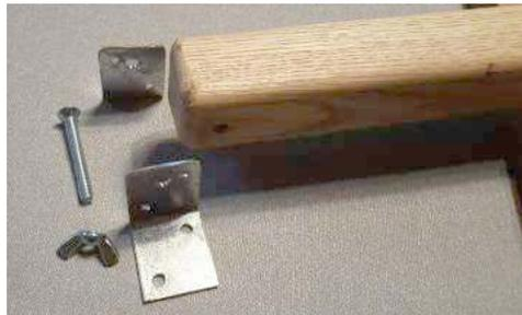
Assemble both brackets to the handle.
