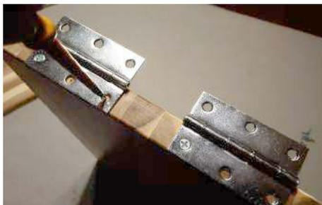
Mark the centers of all the other hinge holes then drill and install the remaining screws.
