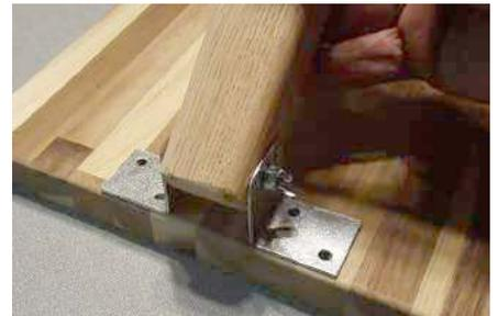
Center bracket assembly on the bottom board. Mark and drill 3/16" holes for the 10-32 x 1" machine screws.
